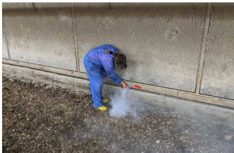
Photo 5: Someone must be inside during the smoke test to identify and mark all locations that are allowing smoke (air) into the building. It usually doesn't take long to figure out where these unexpected air leaks are. We don't expect every surface to be airtight, but we want to take every opportunity to make the building as energy and fuel efficient as possible.
