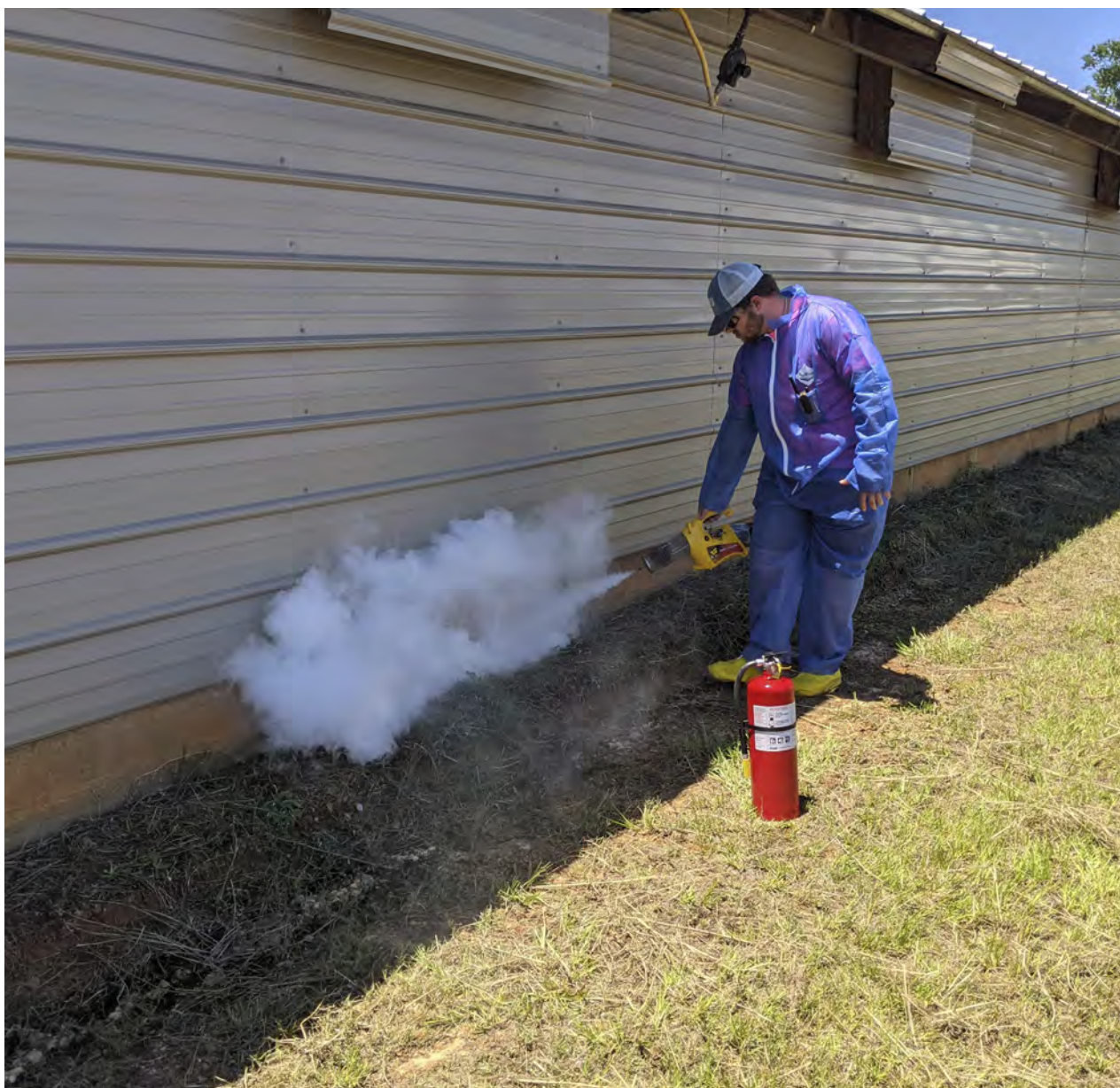
Photo 4: Smoke or fog exterior building surfaces while the house is under pressure to help you identify air leaks that are otherwise hidden from eyesight. Be careful, and keep flames and other hot surfaces away from poultry house materials that may be flammable. Wear PPE and have a fire extinguisher with you as a safety precaution during this exercise.
