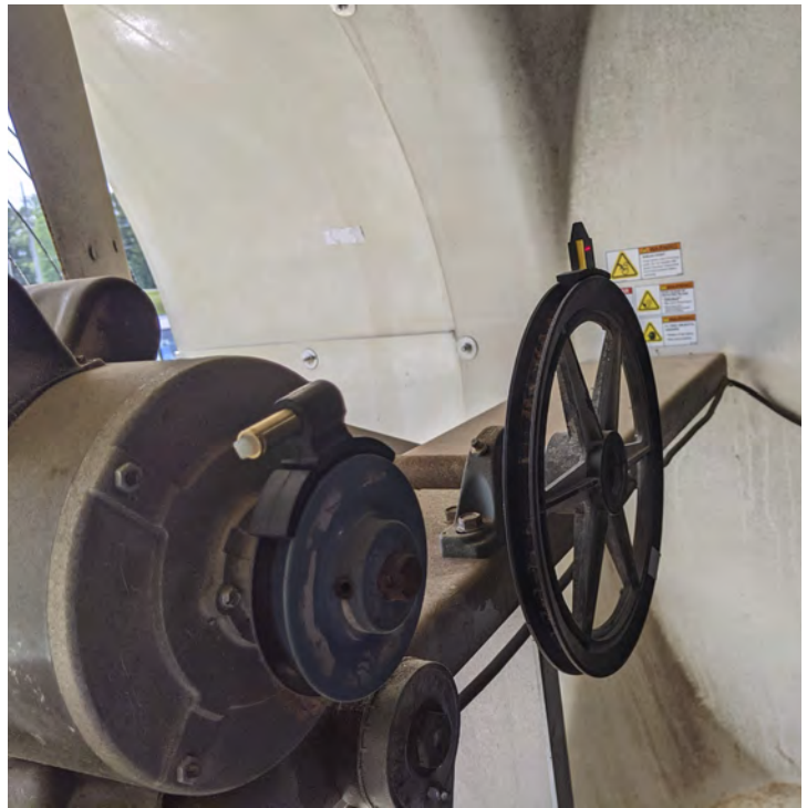
Figure 5: A laser alignment kit is placed on a tunnel fan to evaluate alignment. The laser body is placed on the motor pulley, and the target body is placed on the fan pulley. The laser is hitting to the right of the yellow acceptable band.
