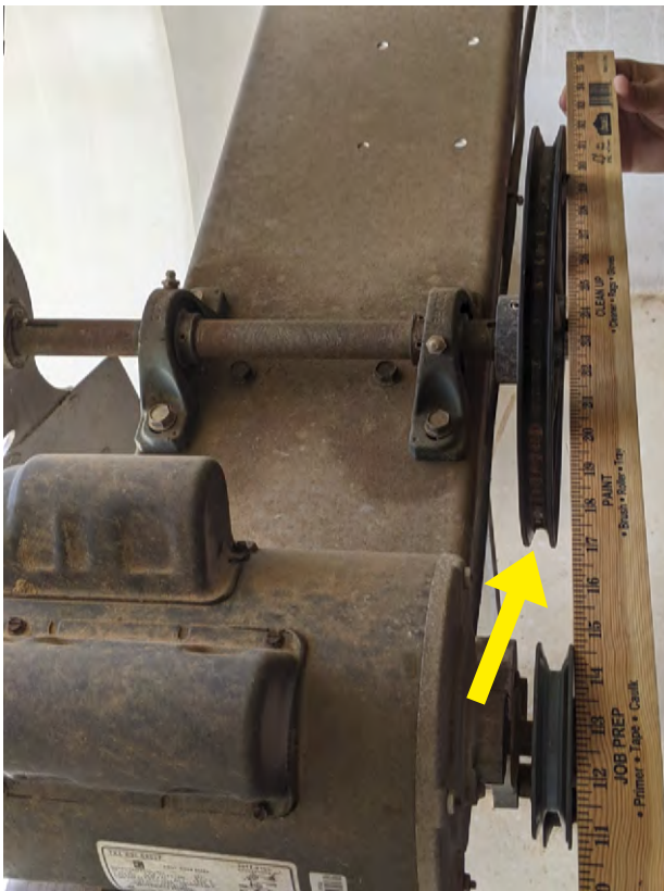
Figure 4: The yardstick method used on a fan where the pulleys are out of alignment approximately 5/8 inch, at left, while, right photo, the yardstick method shows four points of contact and that the pulleys are in correct alignment.
