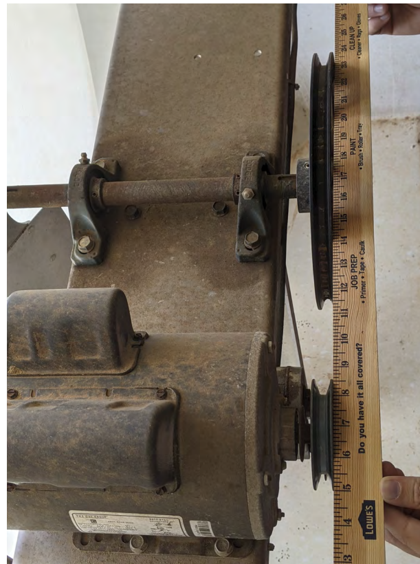
Figure 4: The yardstick method used on a fan where the pulleys are out of alignment approximately 5/8 inch, at left, while, right photo, the yardstick method shows four points of contact and that the pulleys are in correct alignment.
