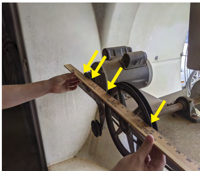
Figure 2: Use a yardstick or something with a straight edge to span across both the fan and motor pulleys. You want to have four points of contact shown by the yellow arrows. Make sure to not lap over the raised area near the shaft, as this will give a false reading.
