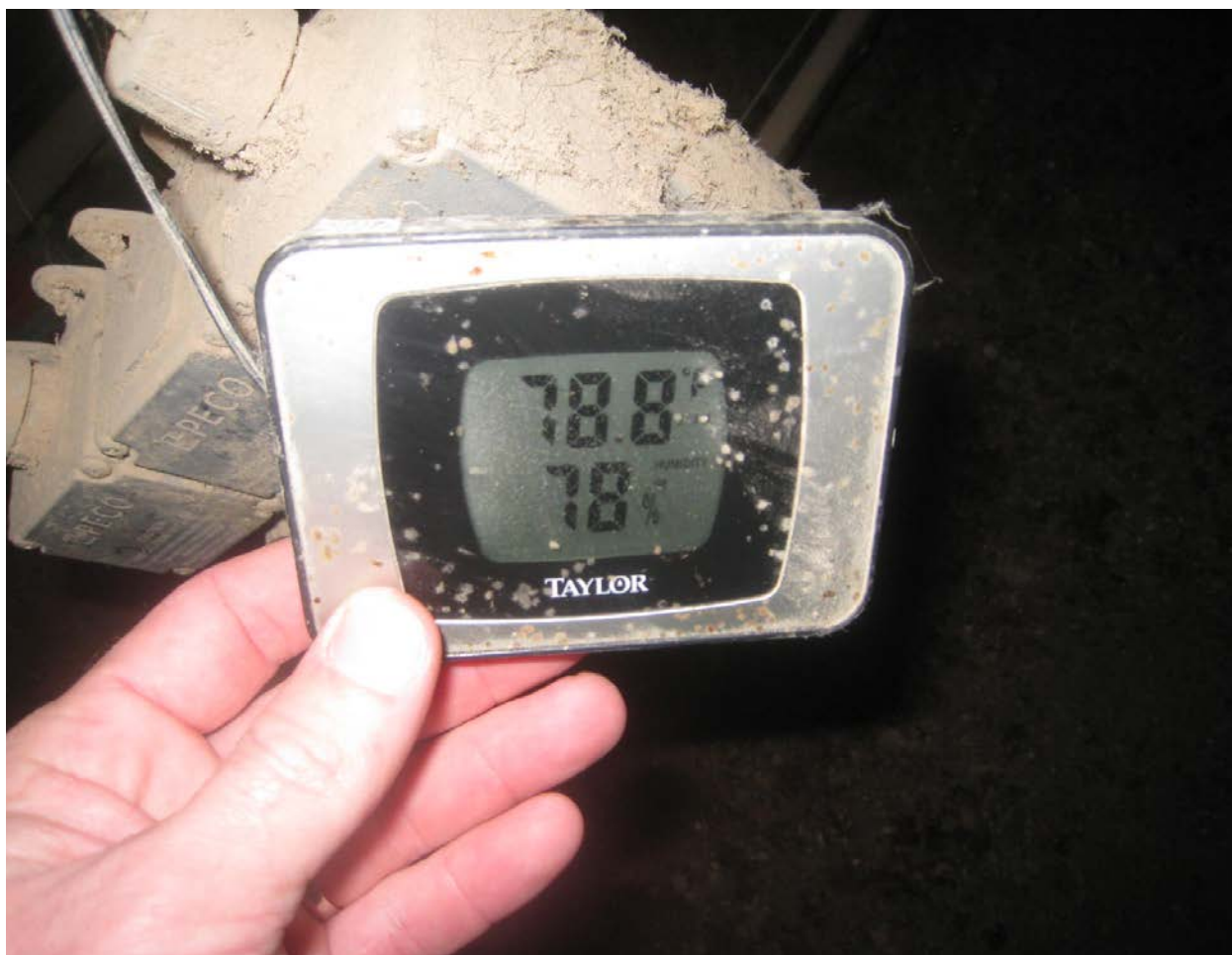
Figure 2: The picture of the relative humidity sensor above indicates the relative humidity inside this house is 78%, which is over the 50-70% ideal range. Corrective action should be taken to lower the in-house humidity by verifying the steps in this article are within parameters, and then increasing fan run times after housing issues are corrected . The ideal time for monitoring relative humidity is in the morning hours, before outside ambient temperature rises.
