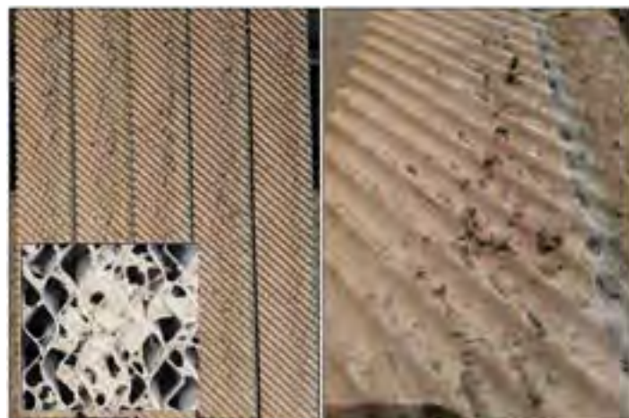
Figure 7: left, pads were pulled out of the system and stacked to demonstrate the debris that is pushed/pulled from the outside surface into the pad flutes. Right, view of the debris lodged midway into a single pad. (Inset, spider webs collecting dirt on the outside surface of a pad.
