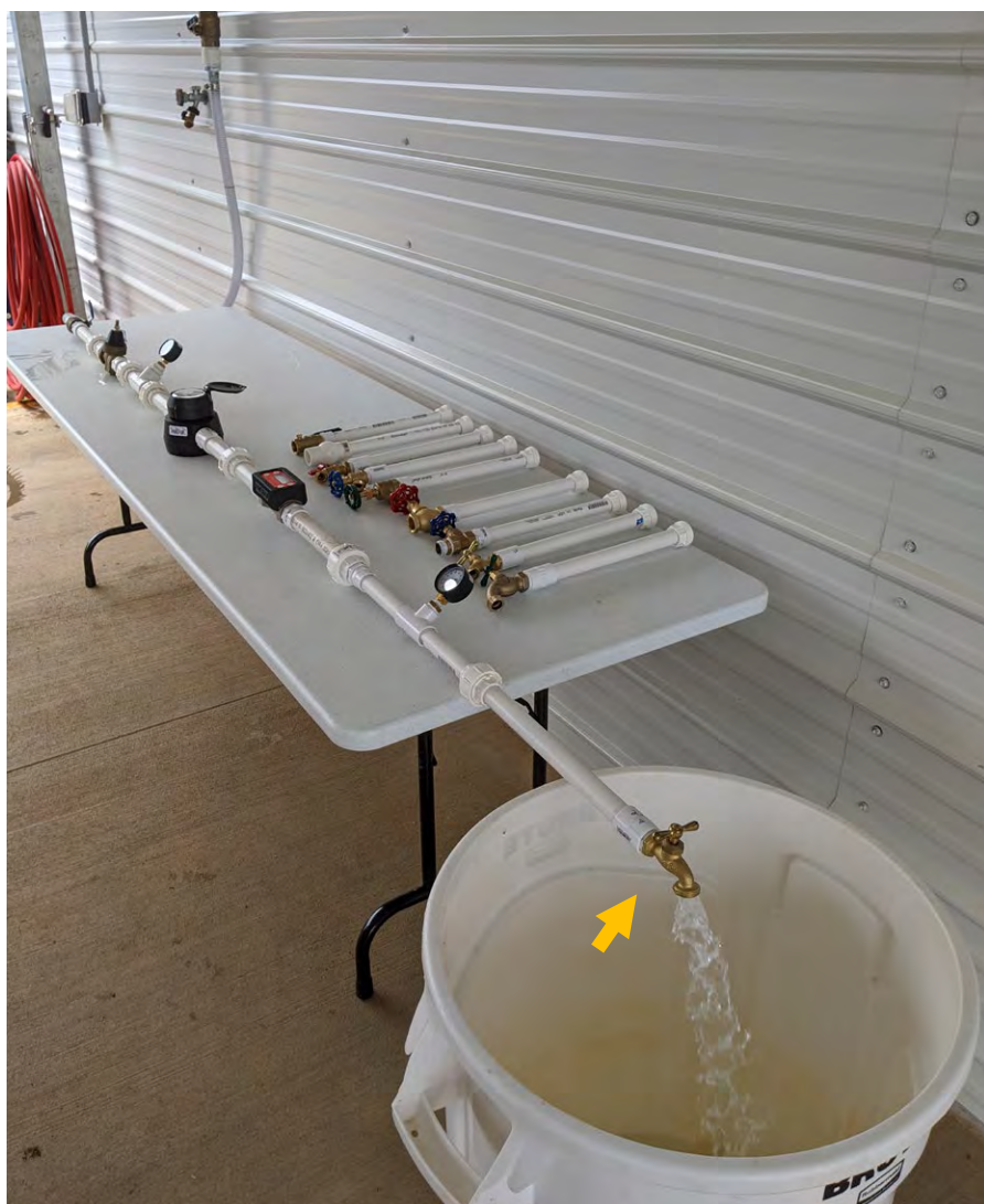
Figure 2: The flow test figure—a flow control valve, pressure regulator, pressure gauge, calibration water meter, digital flow meter, pressure gauge and test valve. Each of the five valves was connected to the union at the end of the table for test. Here, we are testing a brass hose bibb with a supply of 4 gpm (arrow).
