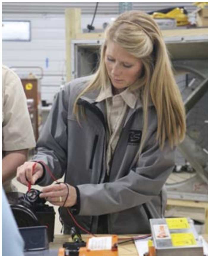
At the 2019 NPTC Breeder Cold Weather Workshop, Logan Dalon, of Tyson-Keystone, is measuring the capacitance of a start capacitor as part of the motor capacitor hands-on training sessions.
